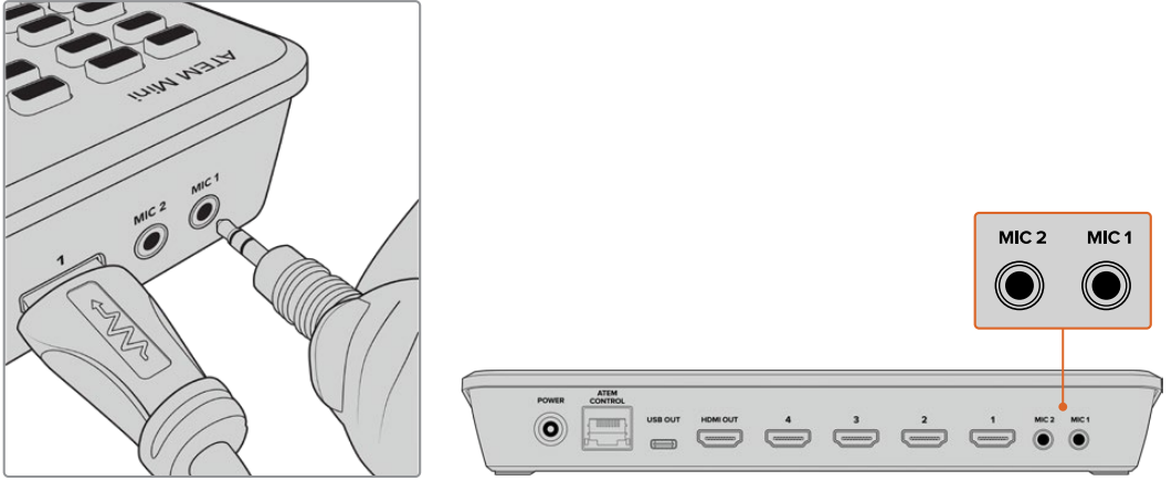
Connect microphones to ATEM Mini's mic inputs
